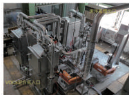
圖二、節能蓄熱式燃燒和吸附濃縮整合系統實體照片 The photograph of the energy-saving adsorption-concentration-and-regenerative-combustion-integration system
