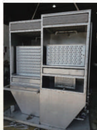
熱泵結合液態除濕系統 Heat pump combined with liquid desiccant dryer
