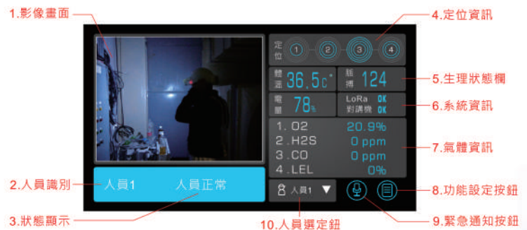
▲後端監控器介面功能區塊說明圖 Illustration of the functional blocks of the remote monitor interface
