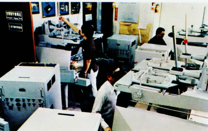
利用蔡司立體製圖儀及錄存儀作模型断面掃描與存錄工作。 Use of Zeiss B 2 Plinimat Plotter with SG-1 Storage Unit for profile scanning and recording.
